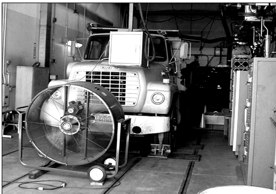
Figure 1. Test vehicle mounted on heavy-duty dynamometer.
